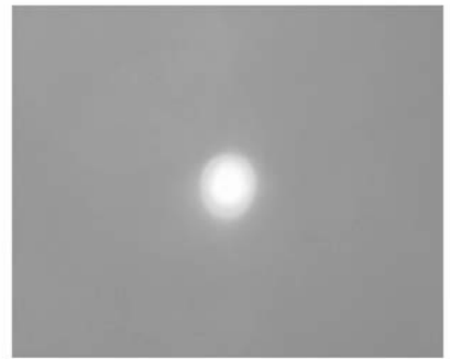
图 6 实验聚焦获得 3 mm × 3 mm 光斑 Fig. 6 Spot size 3 mm × 3 mm after focus lens
